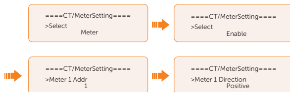
Figure 14-34 Setting meter for the inverter
